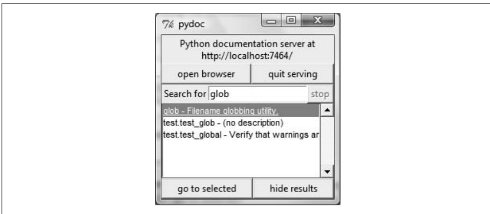
Figure 15-1. The Pydoc top-level search engine GUI: type the name of a module you want documentation for, press Enter, select the module, and then press “go to selected” (or omit the module name and press “open browser” to see all available modules).
